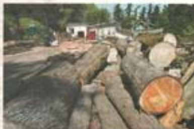
TREES THAT HAVE BEEN SALVAGED are stacked on pallets at Urban Hardwoods, with openings to allow air to flow between the pieces and dry the wood.
